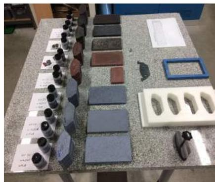
The above pictures show the production process starting with the drawing, the mold and the casted friction pads being glued to the backing plates. (The video showing the die-casting process can be seen at booth #30 at Eurobrake).
